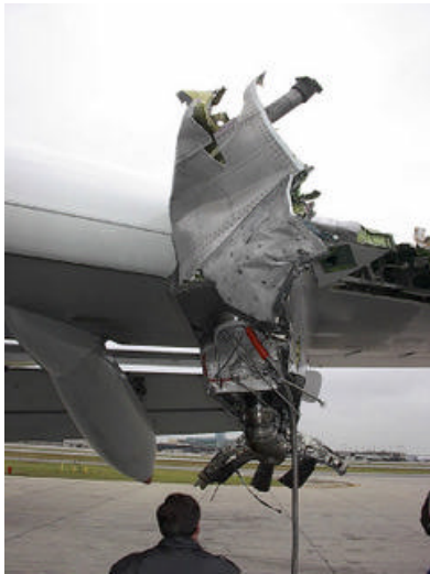
B747 Engine Separation from Mt. McKinley Rotor Encounter
